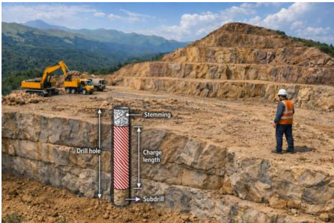
Figure 2.1. Schematic diagram of the borehole configuration used at the Tullallar deposit
