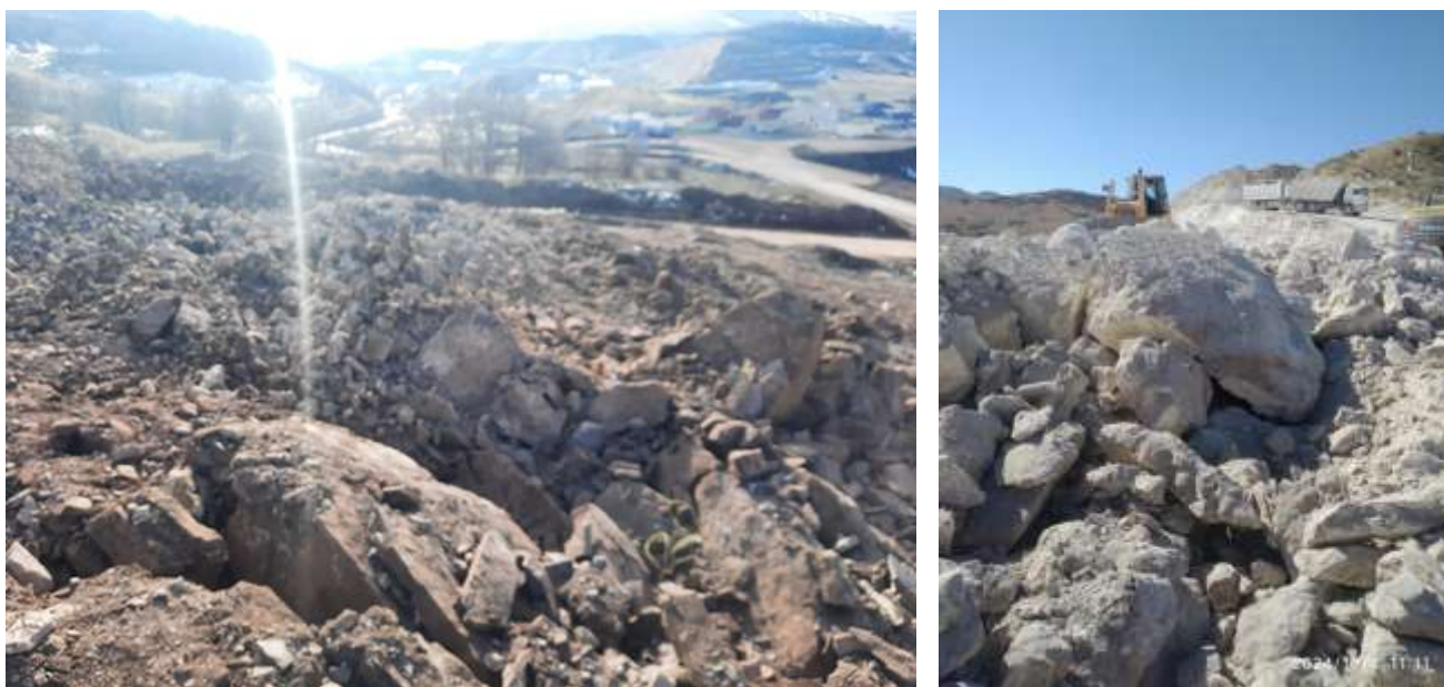
Figure 4.2. Examples of the formation of oversized fragments after mass blasting that require additional secondary breakage: (a) oversized boulders in the muck pile on the bench; (b) large oversized fragments in the muck pile (view under actual quarry operating conditions).
