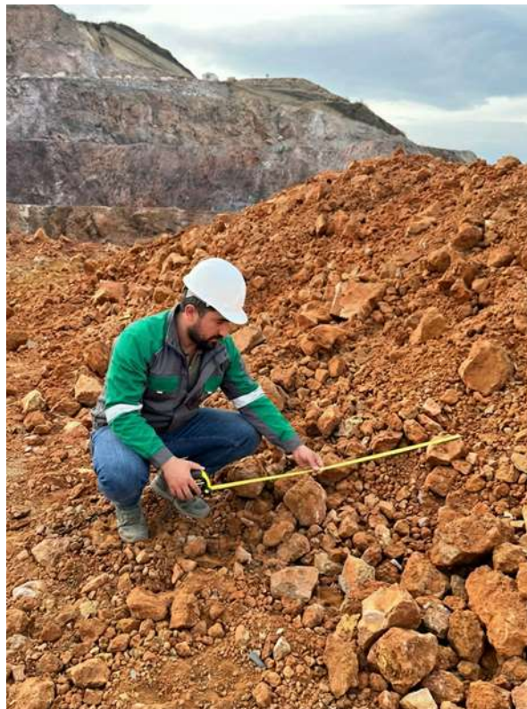
Figure 4.5. Field assessment of the particle-size distribution of blasted rock mass using a reference scale element (measuring tape) for subsequent digital photo analysis in specialized software
