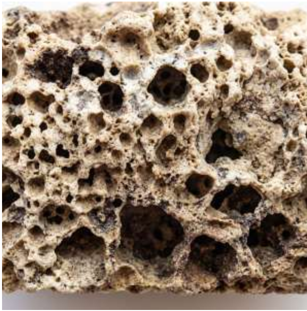
Fig. 2.6. The internal structure of the samples without the addition of chalk.
