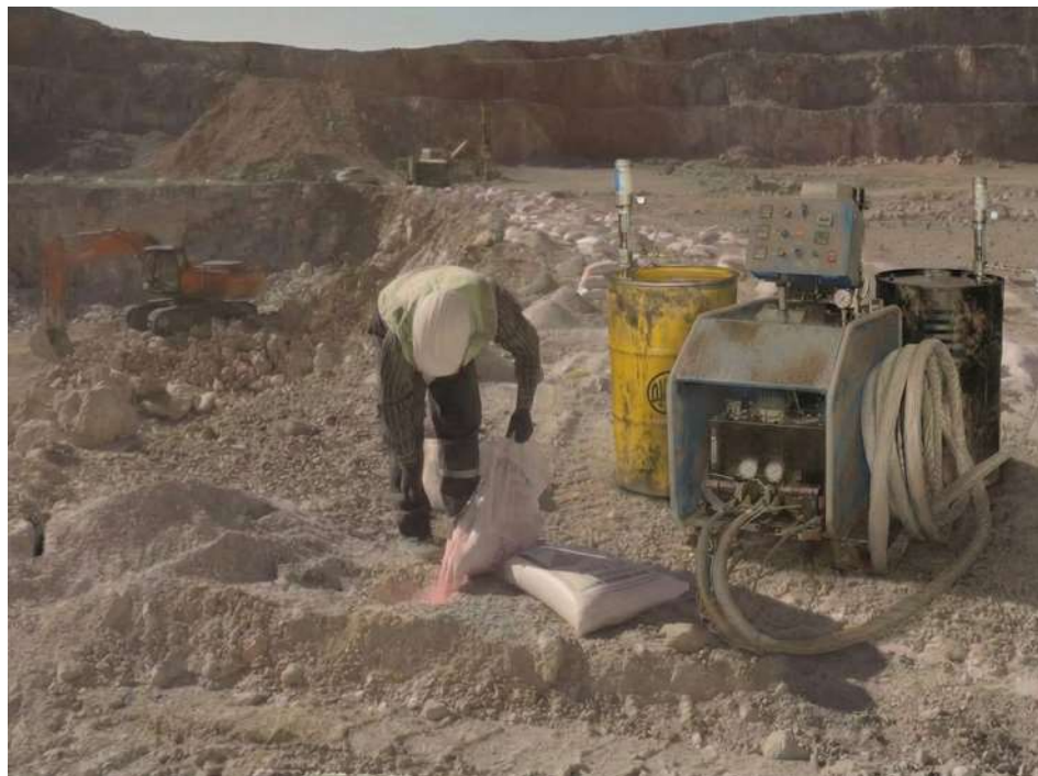
Figure 4.3 Preparation and Application of Foam Stemming under Production Conditions (Foam with Increased Chalk Content) as an Alternative to Sand Stemming
