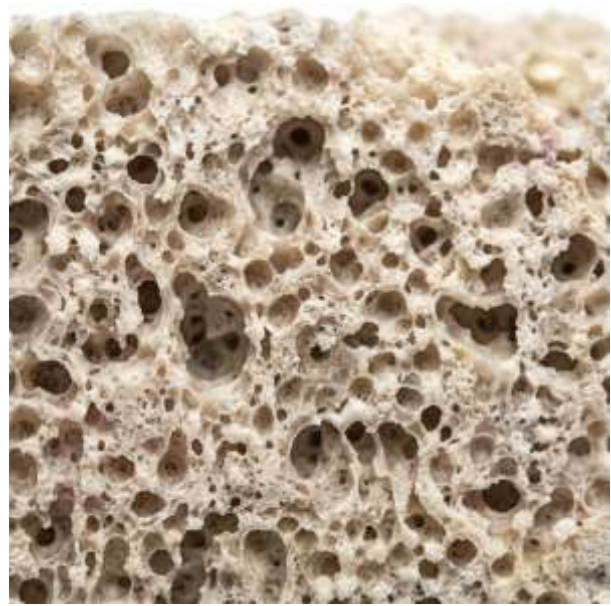
Fig. 2.7. The internal structure of the samples with 5% chalk content.
