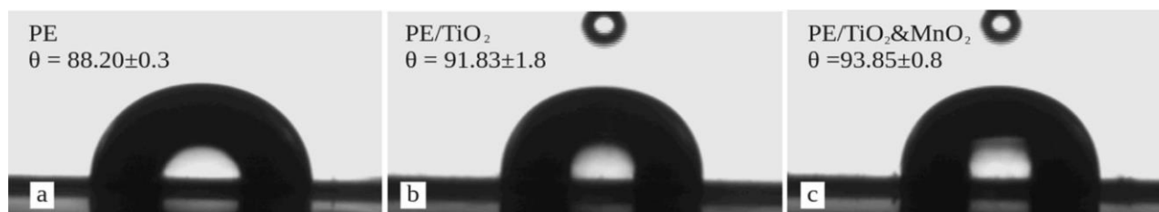
Figure 3.5. Images of water droplets and the corresponding contact angle values just after their deposition on the surface of (a) PE, (b) PE/TiO 2 , (c) PE/TiO 2 &MnO 2 .
