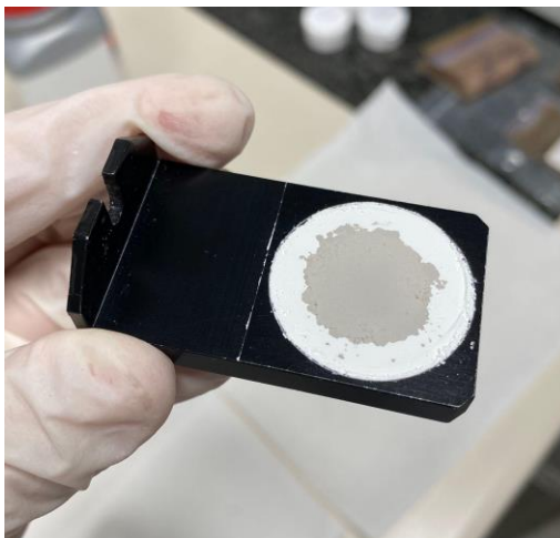
Figure 2.2. Diluted by \text{BaSO}_4 Sample in 12/500 ratio by mass (at the top) placed on \text{BaSO}_4 powder in a metallic holder for DRS measurements.
